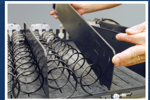
Most trays re-configure to almost any package size in the field with no need for tools.
